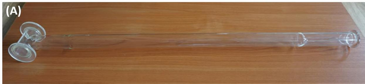
IR cell for adsorption studies at low temperature (100 K)
